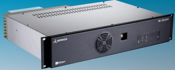
Building on the plug and play principles of analogue Solar 25 simulcast systems, SB2025NT integrated simulcast and voting controller offers enhanced resilience and full remote management of base station network, while interfacing in a cost effective, compact component based P25 system.
